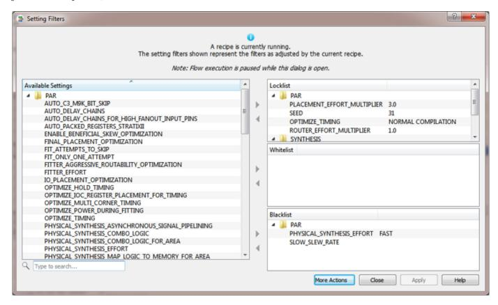
The documentation of each recipe provides details of any changes the recipe makes to the project's setting filters while running (refer to the *Setting Filter Considerations* subsections). Note that any changes made to the project's setting filters by a recipe are reverted when the recipe completes. Use the <code>job summary <job id></code> Tcl command to view the actual setting filters used for a specific job.
