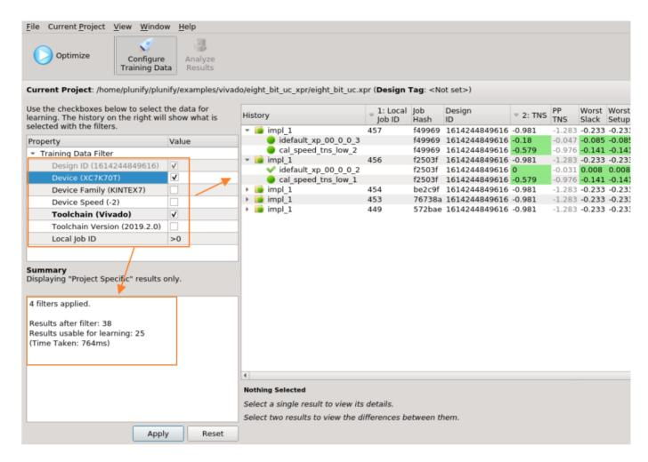
In the GUI, what you see in the history panel is what is being used in InTime's Machine Learning training and prediction. To apply a filter, check the appropriate box or specify a value, then click "Apply". A summary of the number of results left after filtering, and the number of results that are suitable for training and learning will appear.
