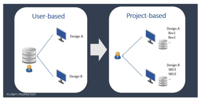
By default, the InTime database for each project is created and stored underneath the FPGA project folder. The advantage is that this enables users to use source revision control, e.g. git, on the database file and have individual database files for different projects. Any user with sufficient file permissions will thus be able to access the database.
