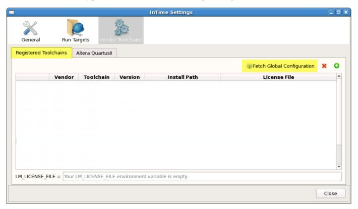
Fetch Global Configuration pulls the information about the FPGA tools that you configured in previous steps. This figure shows many different FPGA tool versions configured in an example setup.
