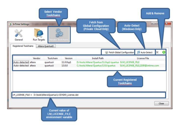
New tools can be added either using the auto-detection mechanism (only available on Windows OS) or the *Register Vendor Toolchain* wizard by clicking on the "Add Tool" button.
