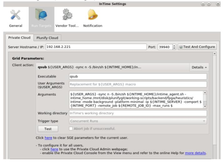
For more information about customizing the grid commands and configuration, please refer to LSF/PBS/SGE/SLURM configuration. Other grids such as SGE and PBS are also supported.
