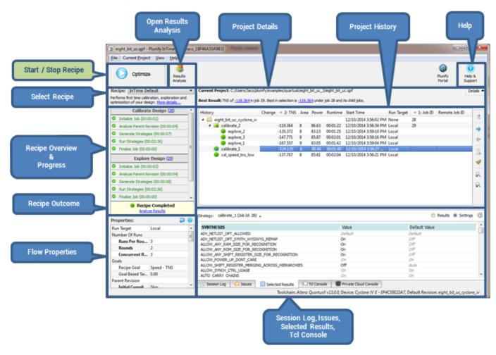
The left side focuses on the active recipe and the InTime flow. The center-right portion focuses on the current project and the section below that provides tabbed panels of details about the active recipe, current project and InTime status.
