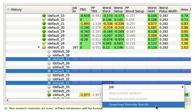
User is able to choose what type of files to download. For report files, check "Results File". For DCP files, check "Proejct File" checkbox. For bitstream files, check "Bit File" checkbox. User is able to overwrite files that were previously downloaded by checking "Overwrite existing files and results" checkbox.
