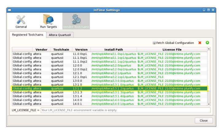
Make sure all the toolchains needed by the Client and build workers are available (Note that they are tagged using the *Global-config* tag in the first column).
