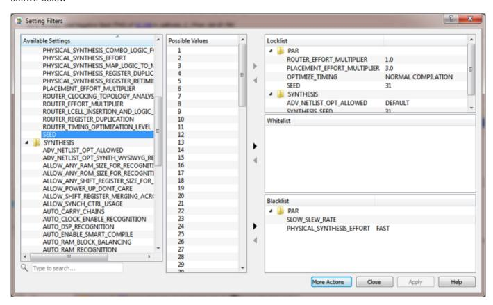
In addition to allowing modification of the project's setting filters, this GUI also allows verification of setting filters and previewing the exploration space for a set of filters.
