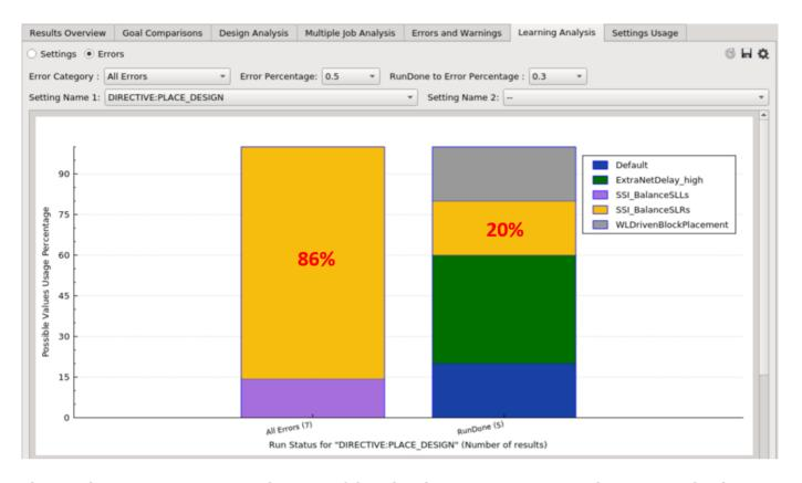
There is also an option to compare the usage of the values between two setting combinations. Each color within a bar represents the possible value combinations between two settings.
